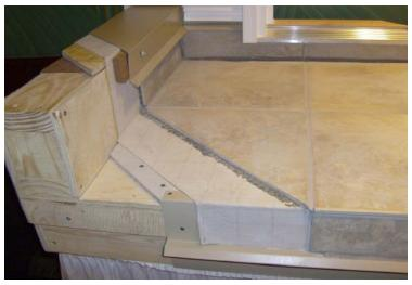
1) Tile Waterproofing Traffic Membrane: Ensurco Duradek Ultra Tiledek; bottom polyester reinforced and polyester top surface PVC membrane with ultra-violet resistance, for fully-adhered installation with heat-welded seams and perimeter attachment designed to receive a tile\* overlay.
